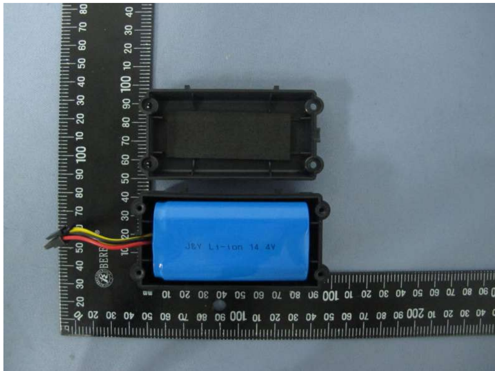
Figure 3 Internal view of battery (内部结构图)
